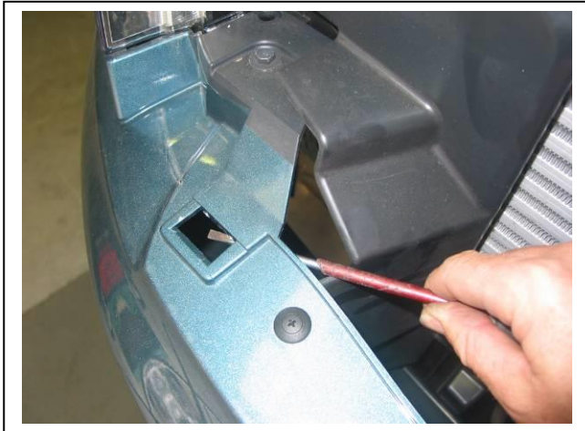
Figure 4: Position of clip with grille removed.
