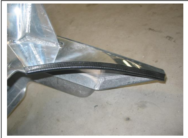
Figure 16: Passengers side clip lock trim fitted
