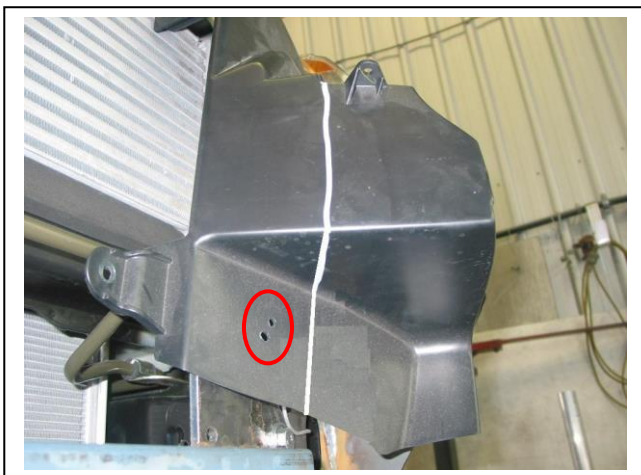
Figure 6: Passengers side air dam trim line and Air sensor positioning shown.
