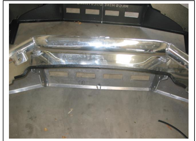
Figure 17: Centre clip lock trim fitted
