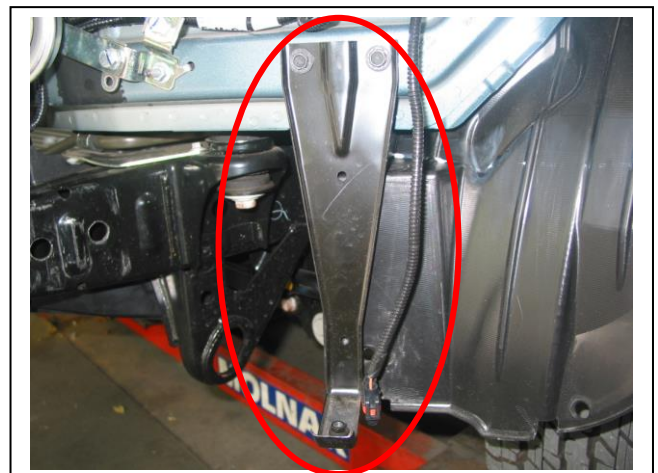
Figure 9: Remove side lower bumper supports. Use removed bolts to fit ECB inner guard supports
