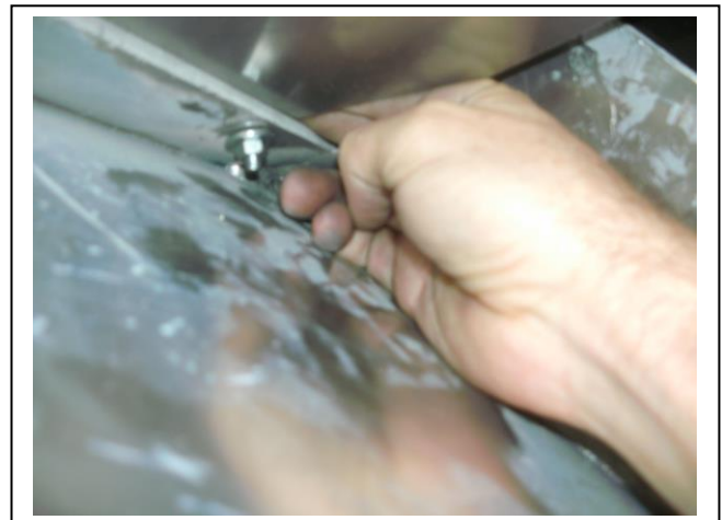
Figure 25: Placing bolt in from side of under body guard.
